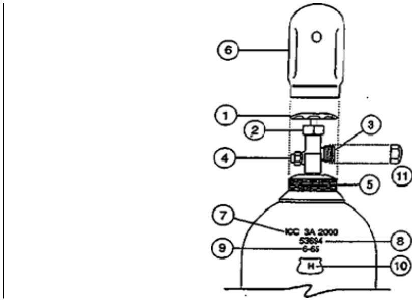
1. Valve handwheel: used to open and close the cylinder valve. Valves are occasionally not equipped with handwheels and require special wrenches to effect operation.
