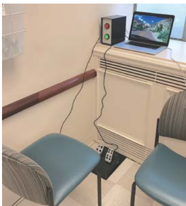
Photograph demonstrating brake reaction time testing setup. Source: Steven Raikin, MD
