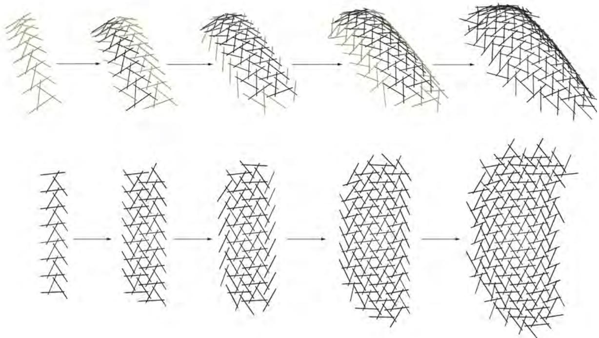
Figure 12: Assembly method of reciprocal structure
