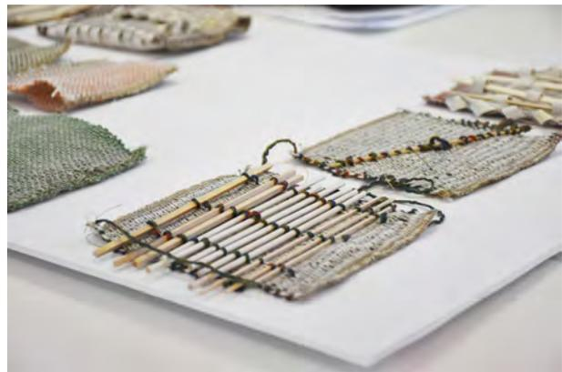
Figure 6: Textile Sample with Integrated Structural Members
