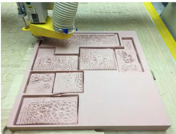
Figure 27: CNC Milling the Facade Iterations
