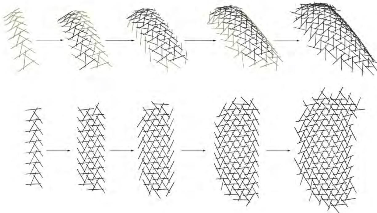
Figure 12: Assembly method of reciprocal structure
