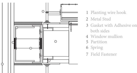
Figure 12: Mullion Mate assembly detail
