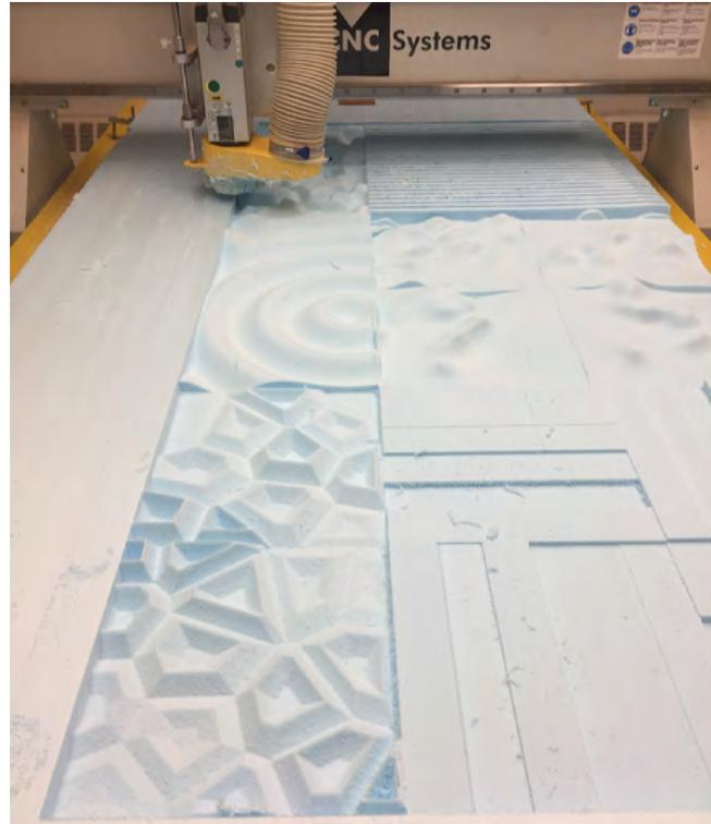
Figure 31: CNC Milling the Mold
