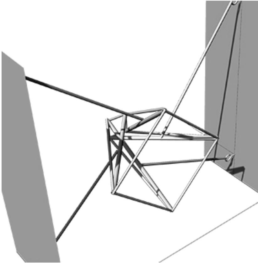
Figure 4: Digital Model showing tensegrity module at rested state
