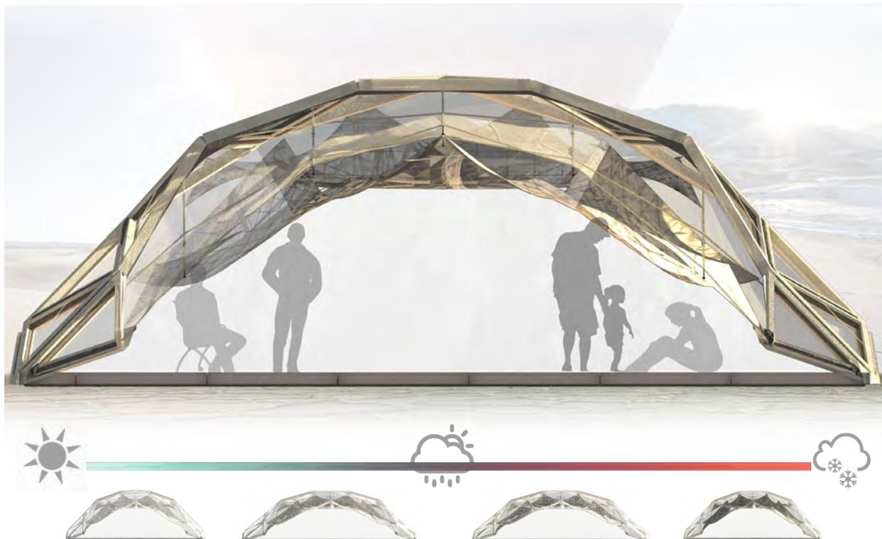
**Figure 15:** Diagrammatic rendering showing different climatic skin conditions .
