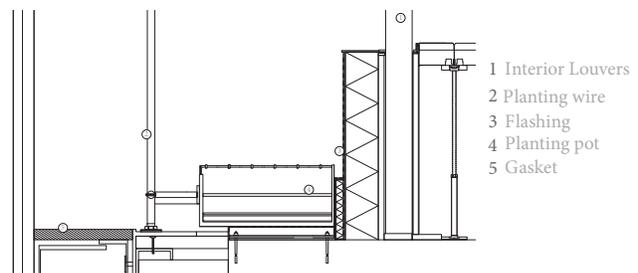
Figure 13: Wall assembly detail
