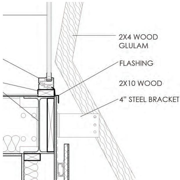
Figure 20: Louver Connection Detail
