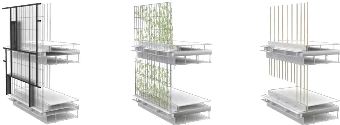
Figure 6: Layers of facade system
