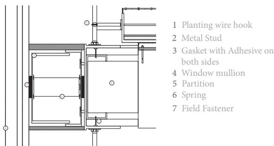
Figure 12: Mullion Mate assembly detail
