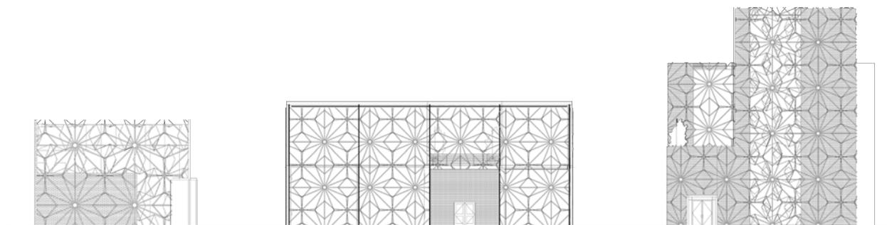
or horizontally along the front face of the glass panels. The exterior screen is bolted at the corners of each individual panel to extensions that come out from the mullions. On Walnut though, the screen is completely detached from the rest of the system and is bolted to the structure grid that hangs out past the facade of the building. All this can be seen in the 1:1 Model in Figure 12 and the Wall section in Figure 13.
