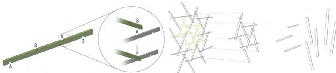
Figure 13: Assembly method of each module within reciprocal structure
