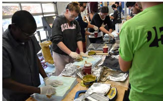
Figure 32: Waxing the Molds
