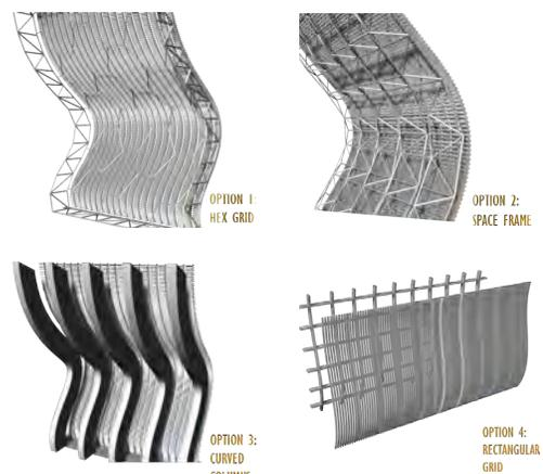
Figure 27: Different Structure Explorations
