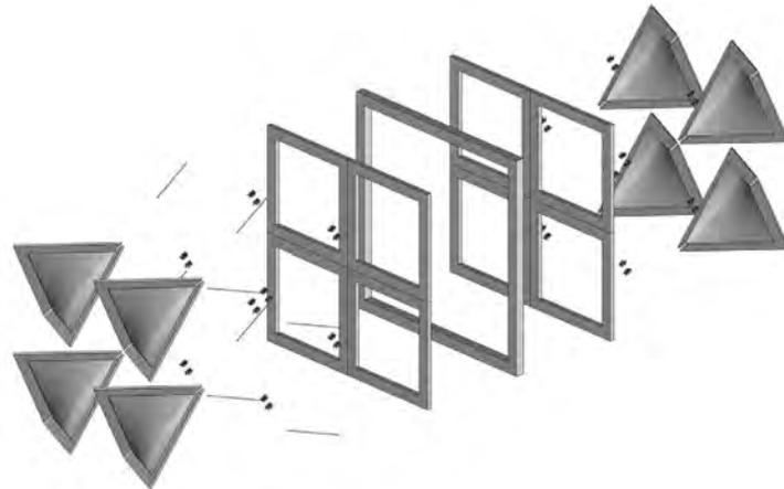
**Figure 14:** Exploded Assembly of Panelized Wind Panel
