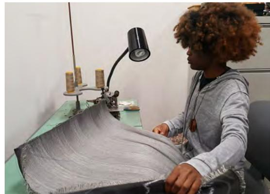
Figure 13: Textile Graduate surging edges of final textile.
