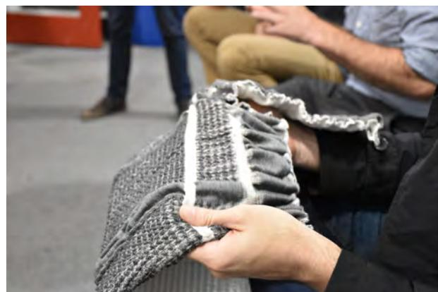
Figure 15: Textile samples weaved on a jacquard loom
