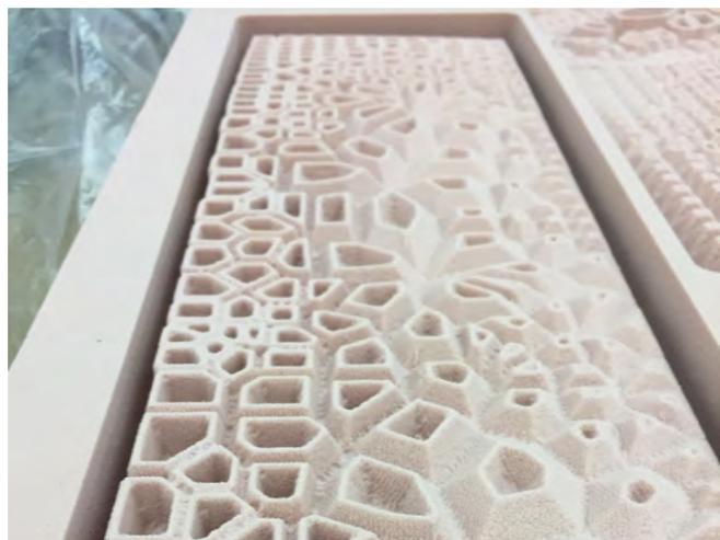
Figure 30: CNC'd Model Foam Facade Representation
