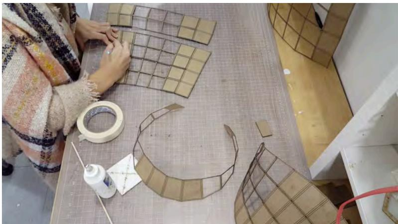
Figure 19: Laser Cut Materials for 1/4" Final Model
