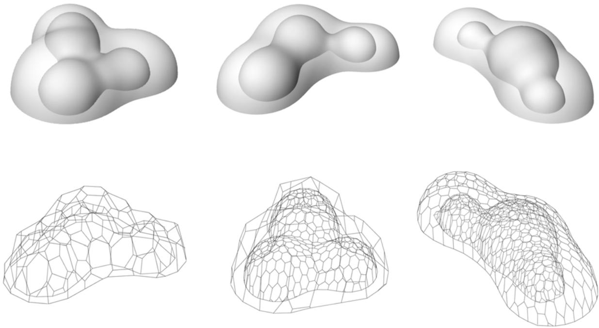
**Figure 5:** Hexagonal pattern mapped to surface
