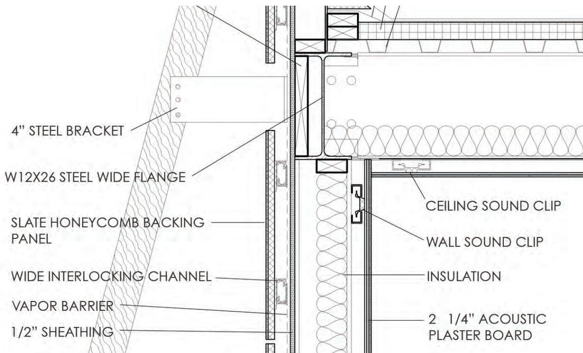
Figure 19: Connection Detail to Soundproof Ceiling and Wall
