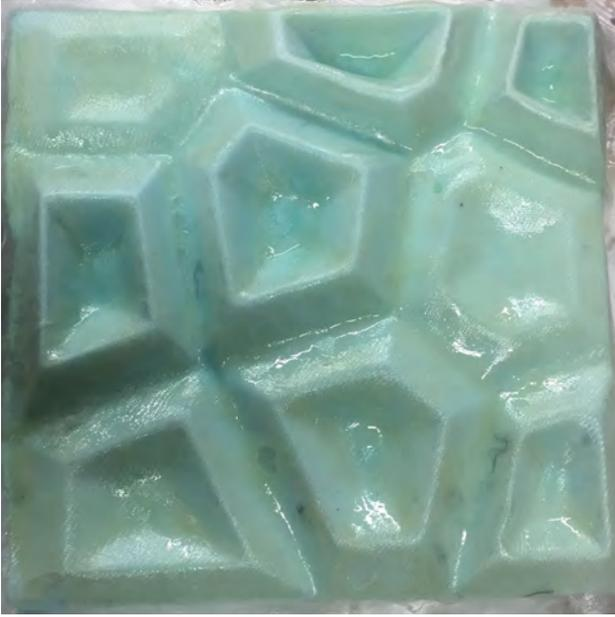
Figure 33: Fiberglass Composite Mold
