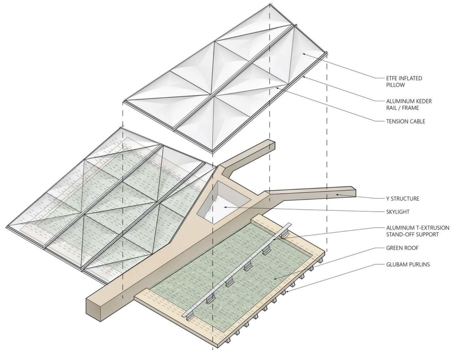
EXPLODED ROOF CONSTRUCTION
