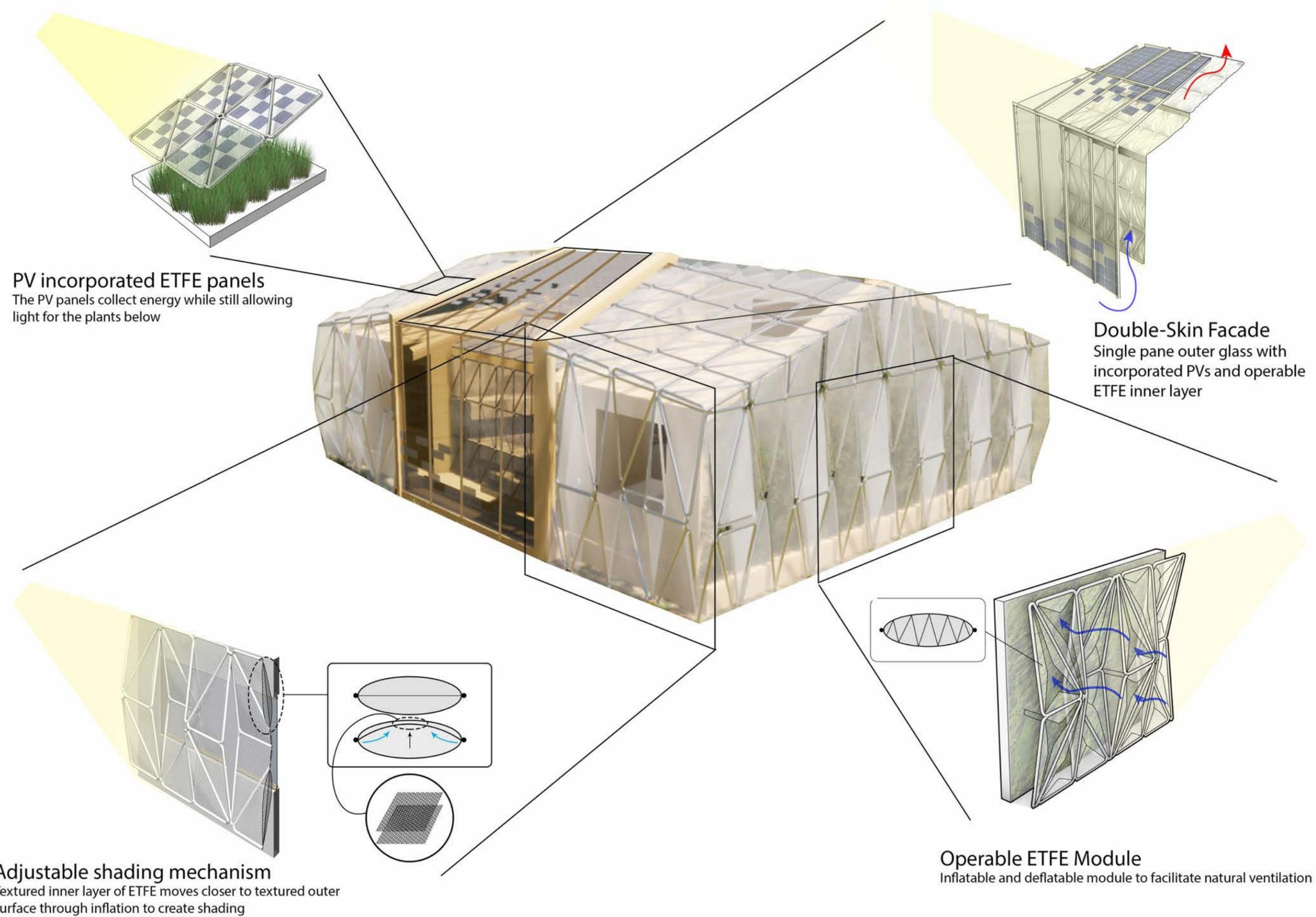
**PV incorporated ETFE panels**
