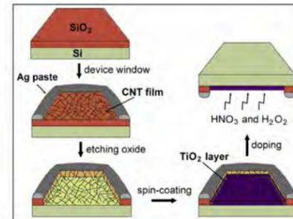
"TiO<sub>2</sub>-Coated Carbon Nanotube-Silicon Solar Cells with Efficiency of 15%"
