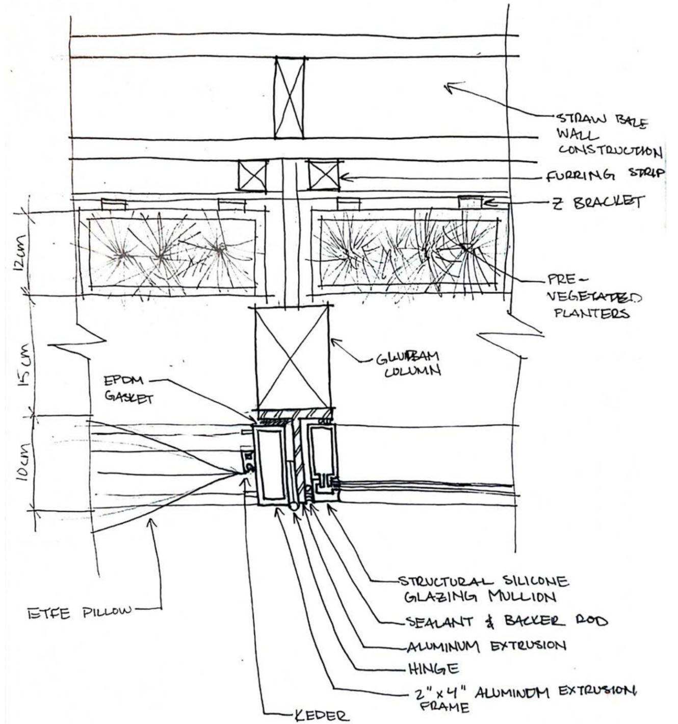
ETFE TO GLASS PLAN DETAIL
