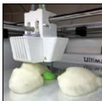
3D kidney model with an upper pole tumor being printed at Jefferson's Health Design Lab facility located at 925 Chestnut Street in the old Federal Reserve vault complex.
