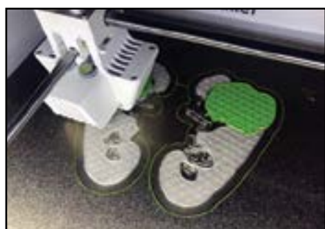
3D kidney model with an upper pole tumor being printed at Jefferson's Health Design Lab facility located at 925 Chestnut Street in the old Federal Reserve vault complex.
