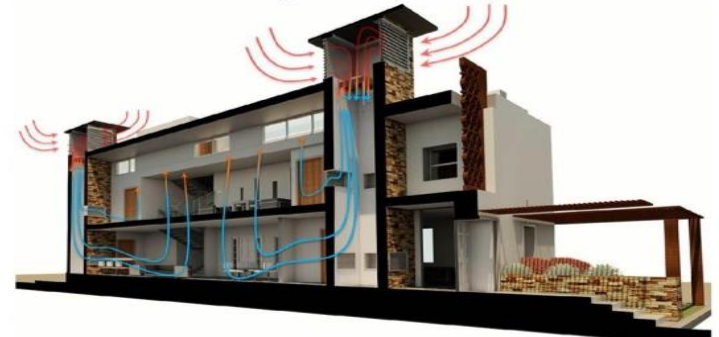
Figure 4-51 3D Section Shows the PDEC through the Family Rooms
